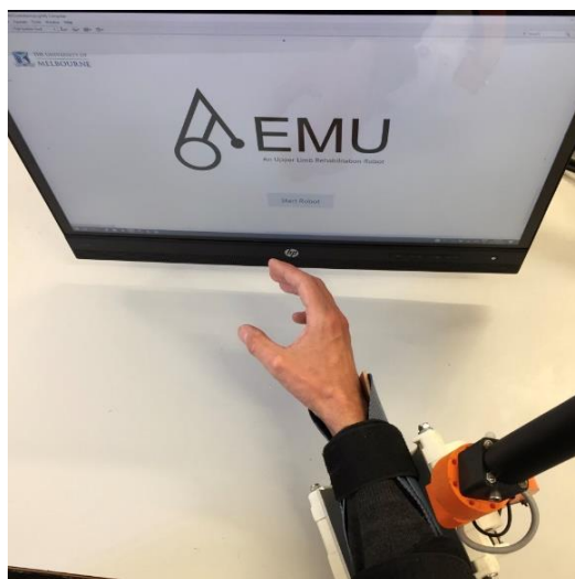
Figure 3 - EMU does not constrain the hand, allowing interaction with the touch screen or real-world objects.
