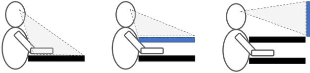
Fig. 1: Types of visuomotor feedback (left to right): Direct: the subject can view their hand directly; Aligned (Indirect): the subject can see a representation of their hand, visually aligned with their physical hand; Unaligned (Indirect) - the subject is presented with a representation of their hand, not visually aligned with their physical hand.
