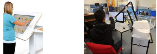
Fig. 3: Examples of one passive device, the Myro (Tyromotion, Graz, Austria) and one robotic device, the EMU [25] with direct visual feedback.
